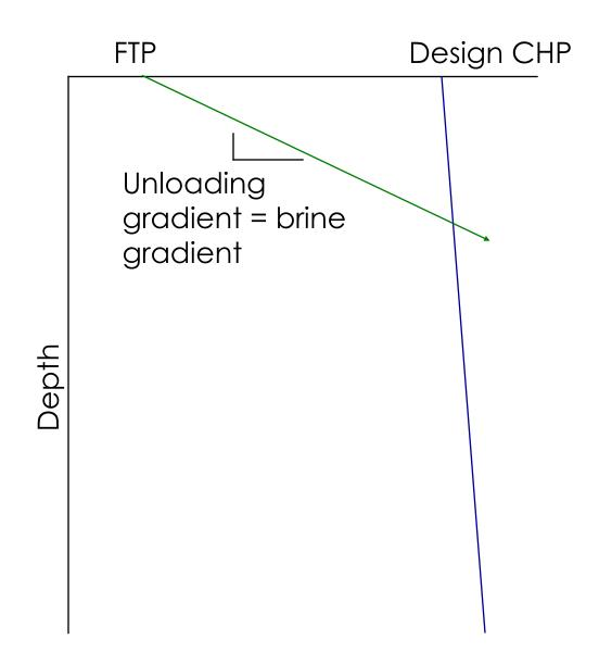
The intersection with the design injection pressure gradient is the top mandrel depth.
