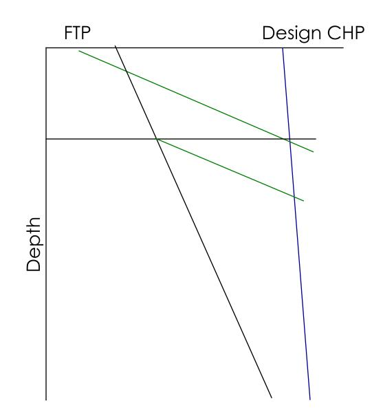
Draw the second mandrel depth where dP exists between the design injection pressure and the unloading gradient. For a system pressure between 1000 and 1400 psi, use dP = 50 psi. Lower system pressures may use less, and higher pressures more.
