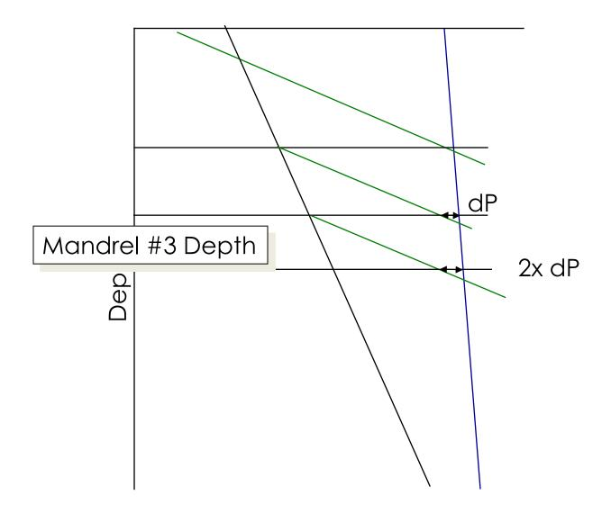
Draw in another unloading gradient. Draw the fourth mandrel depth where 3 times dP exists between the design injection pressure and the unloading gradient.
