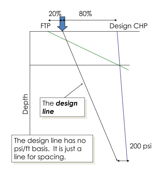
Draw a line at the unloading gradient down from the intersection of the design line to the design injection pressure.
