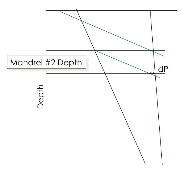
Draw in another unloading gradient. Draw the third mandrel depth where 2 times dP exists between the design injection pressure and the unloading gradient.
