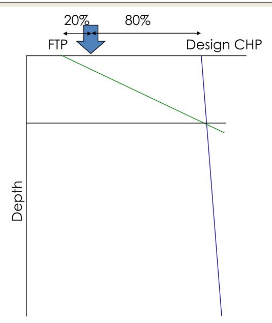
Draw a line down to a point 200 psi less than the injection pressure at the packer (or the perforations, it does not matter).
