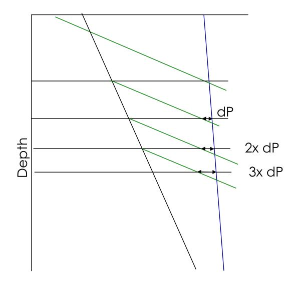
The mandrels are getting progressively close together. We need a minimum spacing or we will end up at the bottom with nothing but mandrels screwed together.
